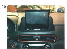
10 Connect all the cables, check the correct operation and put back in place all parts in their position. In the picture it is shown the final result.
