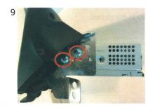
9 Insert the new radio unit as shown in the picture and fix it with 2 M5x8 supplied screws per side.
