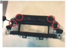
8 Fix the rear plastic shell shown in the picture to the front facia plate with 4 2.9x13 supplied screws as shown in the picture.
