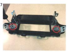
7 Fix the supplied brackets with 2 2.9x13 supplied screws per side as shown in the picture.
